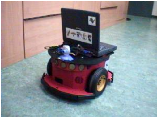
Figure 5: Our pioneer robot with its laptop and camera mounted on (the wireless card is in the laptop)
