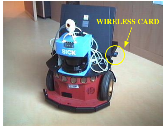
Figure 1: Indoor scenario with 3 access points (left) and our robot with wireless card (right)
